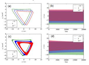
CC BY 3.0 licence (© 2019). Any distribution of this Figure 4: Symplectic conservation test ((a) phase trajectories and (b) amplitude are calculated by the symplectic in-∉ tegral algorithm; (c) and (d) are results using equation (4)).
