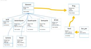
Figure 1: Li-track overall structure (blue arrows represent derivative relationship, and yellow arrows represent calling relationship).
