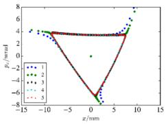
Figure 2: The phase trajectories calculated by Li-track under different integral step sizes (k=1,2,3,4,5).
