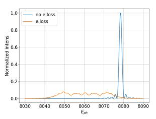
Figure 4: Normalized undulator radiation intensity with and without energy loss.
