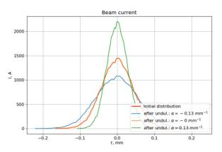
Figure 2: Beam current after THz undulator.
