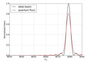
Figure 5: Normalized undulator radiation intensity with and without quantum fluctuations. 15 undulators with number of periods 125 each.
