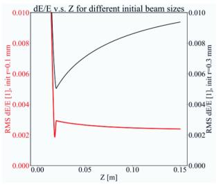
Figure 8: Energy spread for bunch radius 0.3 mm (black) and 0.1 mm (red).
