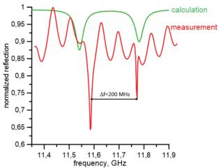
Figure 9: Measured (red) and calculated S<sub>11</sub> parameters.
