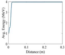
Figure 6: Energy of particles accelerated in gun resonator.
