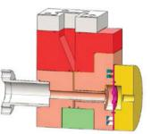
Figure 1: 11.7 GHz RF gun engineering design.
