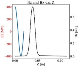
Figure 5: Longitudinal E-field distribution and Bz field distribution.
