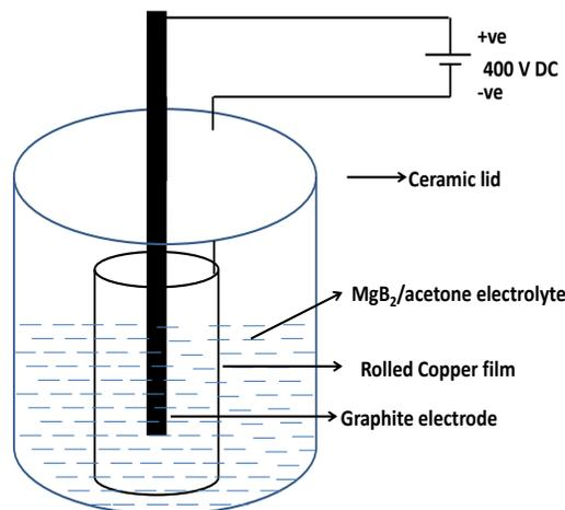
Figure 1: Set up for room temperature electrochemical deposition of  $MgB_2$ .
