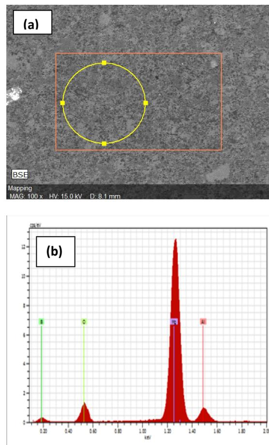
Figure 3: (a) SEM analysis of magnetron sputtered  $MgB_2$  thin film and (b) EDX analysis  $MgB_2$  thin film.
