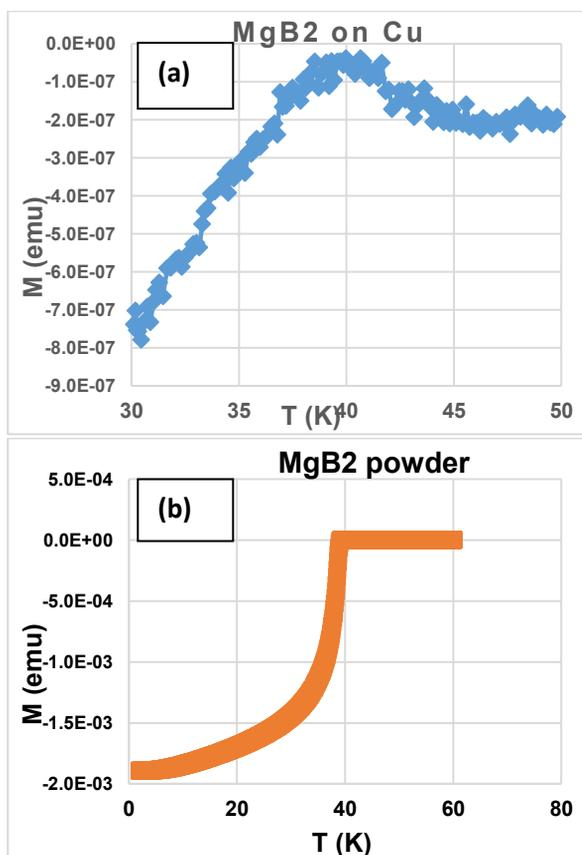
Figure 2: DC Magnetisation as a function of temperature a)  $MgB_2$  deposited on copper and b) as received  $MgB_2$  powder.
