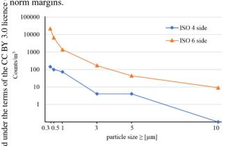
Figure 4: Measured particle concentrations during roll-up g door operation inside the lock (ISO 4) and on the ISO 6 side.
