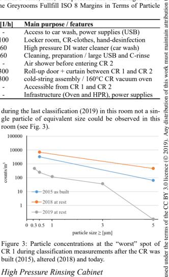
Figure 3: Particle concentrations at the "worst" spot of CR 1 during classification measurements after the CR was built (2015), altered (2018) and today.
