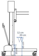
Figure 5: Left: Photo of the lift trolley handing over a cavity in its frame to the lifter system of the ultrasonic bath. Picture was taken during the testing of the cleanroom infrastructure with a 3 GHz cavity from TU Darmstadt [20]. Right: Sketch of the probe positions during particle measurements without cavity.
