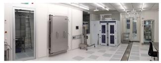
Figure 2: Photo of CR 2: the HPR with its lever for the movable wand (on top) is shown. The door of the vacuum oven and a lift trolley is shown as well.
