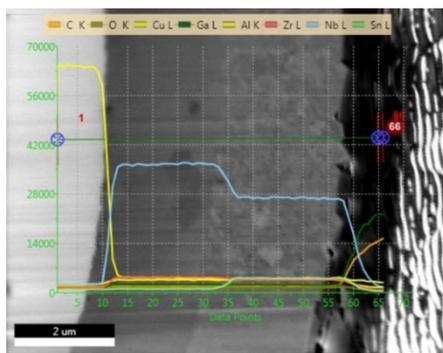
Figure 4: EDX line scan of homogeneous area of sample A15-4.
