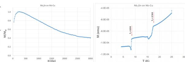
Figure 5: Normalized dc magnetization curves as a function of external applied field (left) and magnetization as a function of temperature (right) for Nb<sub>3</sub>Sn/Nb bilayer film deposited on copper for sample A15-4.
