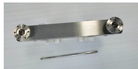
Figure 1: prototype stripline kicker
