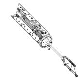
Figure 3: Mechanical schematic of CSNS wire scanner.
