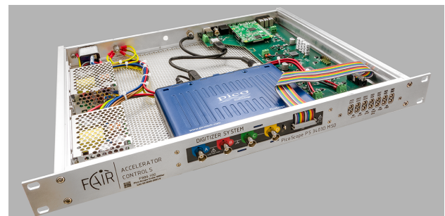
Figure 1: GSI-designed integration of PicoTech's PS3000-series digitizer into a rugged 19"-1U form-factor.
