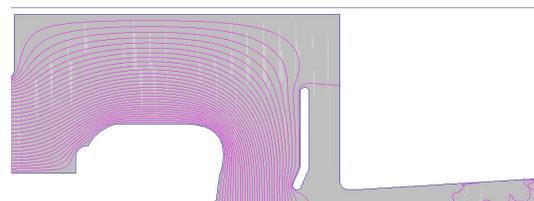
Figure 5: The geometry of the selected electron gun.
