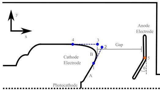
Figure 3: A sketch of the electrode parameterisation. The cathode control points are marked in blue. The dashed dark blue lines show when points are in line. The point where the angled section of the anode begins is marked in orange. The black dashed line is the axis of rotational symmetry.
