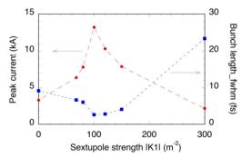
Figure 8: Simulated bunch profile tuning by the sextupole magnets.
