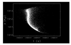
Figure 7: Simulated energy-time phase space plot at the BC2 exit of the SACLA-BL1.
