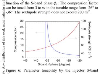
Figure 6: Parameter tunability by the injector S-band phase.
