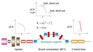
Figure 1: Concept of the nonlinear energy chirp correction using sextupole magnets.
