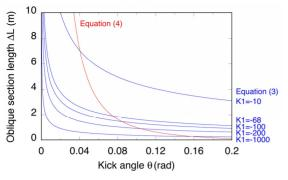
Figure 5: Chicane parameter conditions for various sextupole strengths.
