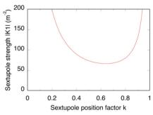
Figure 4: Sextupole strength as a function of the position factor k.
