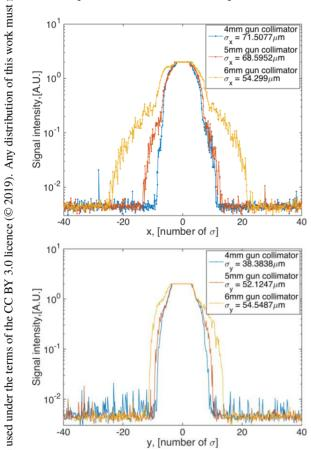
Brigure 2: Horizontal (top) and vertical (bottom) beam halo distribution measured after linac and before CL
