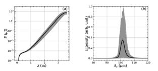
Figure 4: (a) THz pulse energy along the undulator and (b) its spectrum at the exit.
