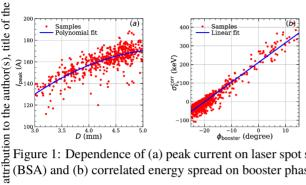
Figure 1: Dependence of (a) peak current on laser spot size (BSA) and (b) correlated energy spread on booster phase.
