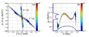
Figure 3: (a) Transverse and (b) longitudinal phase spaces at the undulator entrance.
