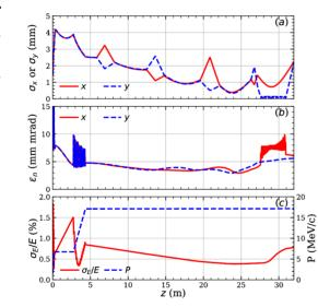
Figure 2: Start-to-end simulation: (a) rms beam sizes, (b) momentum along the beamline. normalized emittances and (c) rms energy spread and mean
