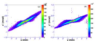
Figure 6: Measured transverse phase spaces in (a) horizontal and (b) vertical planes:  $\varepsilon_{n,x} = 4.0$ ,  $\varepsilon_{n,x} = 3.8$  mm mrad.
