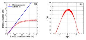
Figure 5: Measurement of (a) emission curve and (b) bunch profile.
