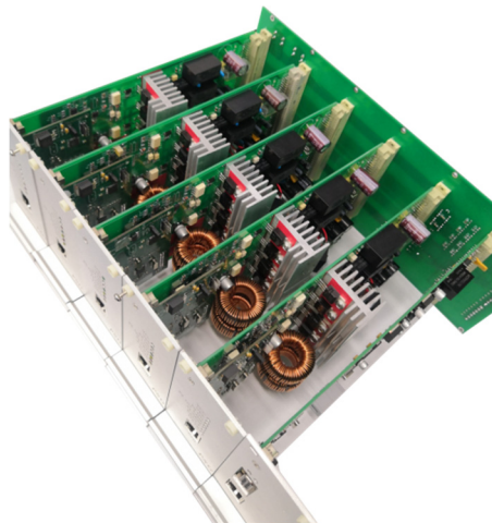
Figure 5: Internal structure of the power supply.
