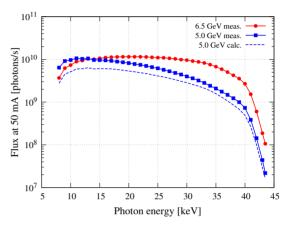
Figure 5: Comparison of SR spectra at NW10A between the 6.5-GeV and 5-GeV operations. The dashed line shows the calculated estimate.
