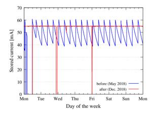
this work must maintain attribution to the author(s). Figure 4: Stored currents of the PF-AR before and after introducing the top-up injection. The current is maintained at  $55 \pm 0.1$  mA after the introduction, while it is topped up uo three times a day to 60 mA before. The current drops in distributi the figure are due to beam dumps caused by machine issues or re-injections for recovering the sudden drop of the beam Flifetime.
