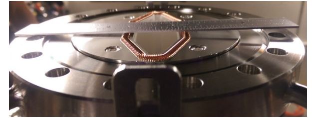
Figure 4: Flange image of the bellows with trapezoidal groove and the RF contact spring at place after disassembling.
