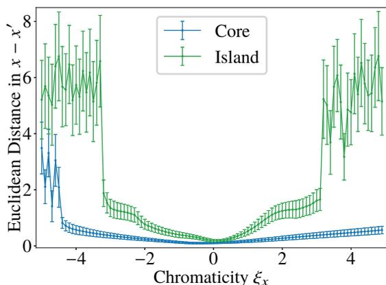
Figure 5: Euclidean distance between two particles with identical transverse starting coordinates but different momenta averaged over 1000 turns as shown in Fig. 4 as a function of the horizontal core chromaticity  $\xi_x$ . [6, 9]
