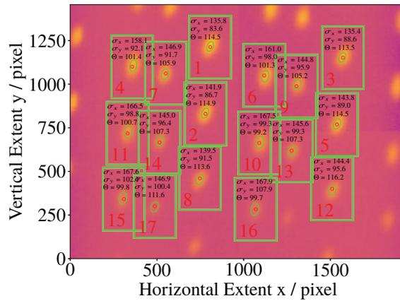
Figure 1: Image at pinhole 9 with TRIBs optics and all current on the second orbit. Three spots correspond to one pinhole. Coupling [5] gives vertical separation of the beam spots for the horizontal resonance. The ROI's are found in order of the peak height and numbered accordingly. [6]
