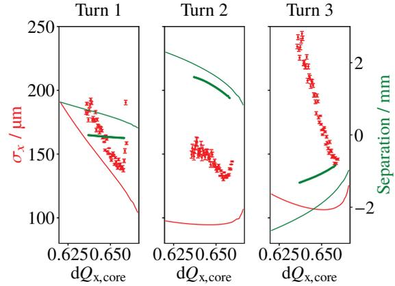
Figure 3: The simulated (red lines) and measured (red dots) transverse beam sizes  $\sigma_x$  at Pinhole 9 as a function of the fractional horizontal core tune  $dQ_{x,\text{core}}$  together with the corresponding separation (green). The simulation is based on our measured linear optics from closed orbits and nonlinear optics fitted to match the chromaticity and tune shift with amplitude measured at the machine in 2018. [6, 9]
