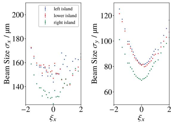
Figure 6: Transverse beam size measured at pinhole 9 as a function of the horizontal core chromaticity. The intermediate steps of the chromaticity rely on the accuracy of the BESSY II chromaticity bump. It was also measured directly at the beginning and end of the scan. [6]
