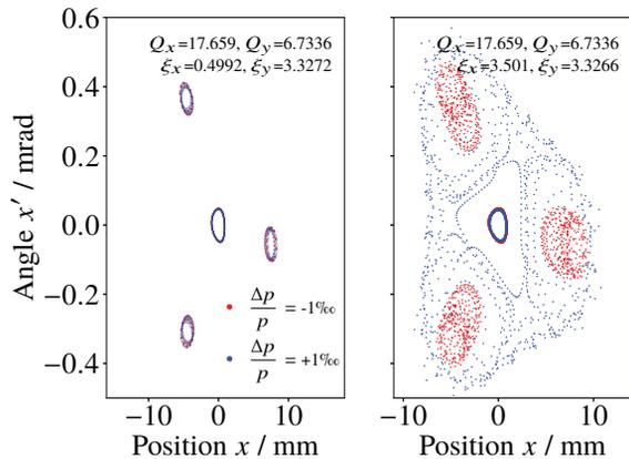
Figure 4: Trajectory of particles with initially identical transverse coordinates  $(x, x')$  but different initial momenta ( $\delta = \pm 1\%$ ) at  $\xi_x = 0.5$  (left) and  $\xi_x = 3.5$  (right) over 1000 revolutions. [6, 9]
