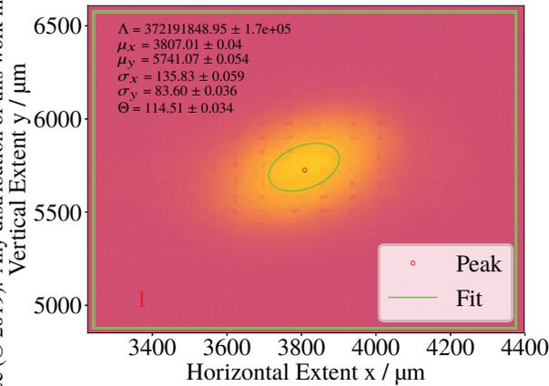
Figure 2: Exemplary fit of a 2D rotated Gaussian function to the beam spot in ROI 1 in Fig. 1. [6]
