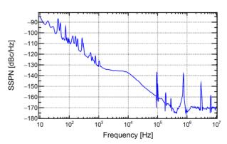
Figure 3: Cavity phase noise spectrum at ELBE.
