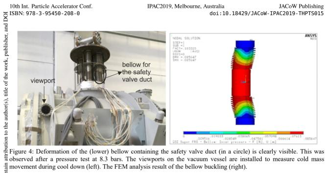
movement during cool down (left). The FEM analysis result of the bellow buckling (right).
