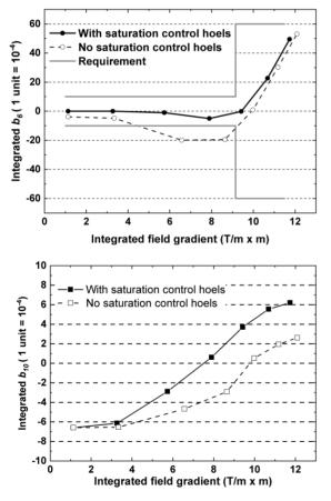
Figure 2:  $b_6$  as a function of integrated gradient (top). The solid lines indicate the field quality requirement.  $b_{10}$  as a function of integrated gradient (bottom).
