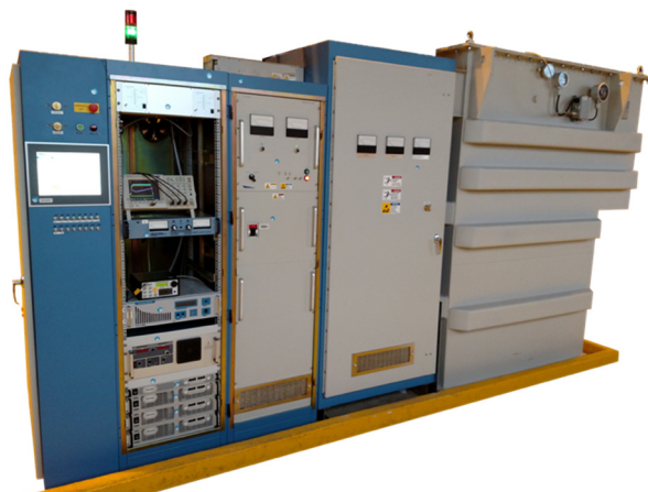
Figure 1: ESS Klystron Test Stand, showing controls and auxiliary supplies in the left cabinet, the high voltage power supply (center-left), the high voltage modulator cabinets (center-right), and transformer (far right).
