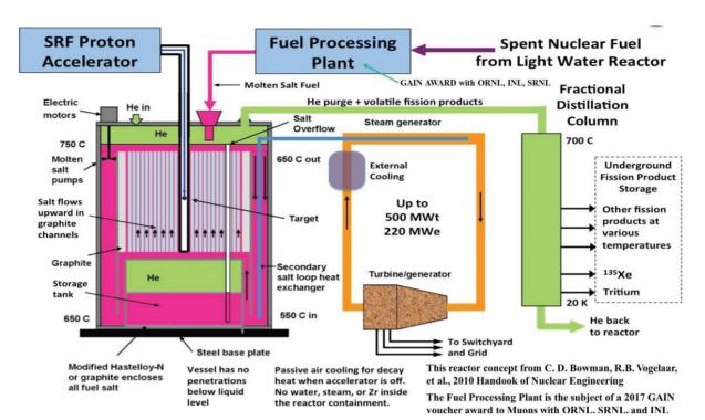
Figure 1: Conceptual diagram of the Mu\*STAR system, comprised of a 1 GeV, 2.5 MW SRF proton Linac, a 500 MWt graphite moderated reactor with internal solid metal spallation neutron target, a molten-salt fuel preparation plant, and 5 collection system for volatile radioisotopes. The reactor power can be used for process heat or electricity generation.
