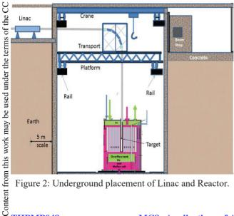
Figure 2: Underground placement of Linac and Reactor.
