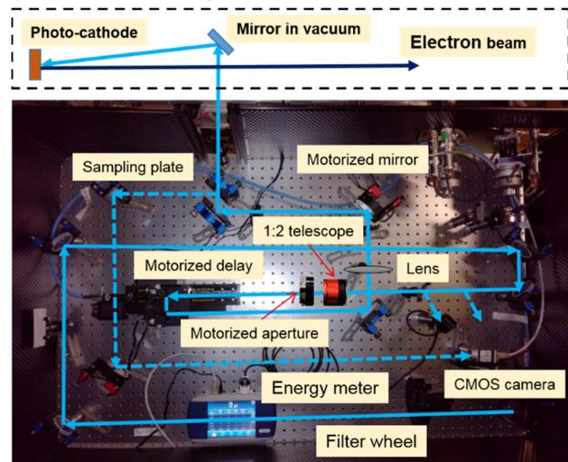
Figure 4: Virtual cathode setup. The light-blue lines show the UV beam path starting from the 1<sup>st</sup> mirror in the right bottom corner up to the photocathode. The reference beam path from a sampling plate to the CMOS camera is shown by the dashed light-blue lines. Elements inside the vacuum system (in the dashed rectangular) are shown schematically.
