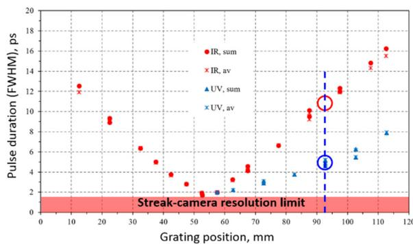
Figure 2: Duration of IR and UV pulses in the secondary laser beam as a function of the second diffraction grating position in pulse compressor II.
