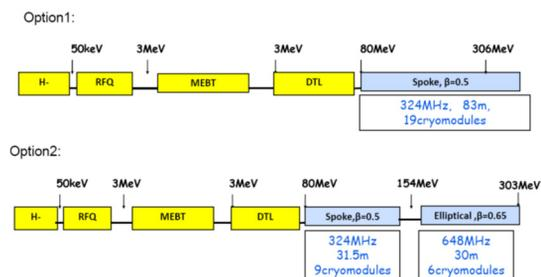
Figure 14 : Two options of the S.C. linac.
