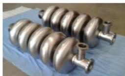
Figure 16 : S.C. elliptical cavity developed at IHEP.
