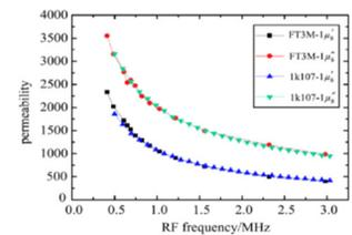
Figure 17 : Measurement(upper) of the domestically developed MA strip and its results(lower) in comparison with HITACHI products FT3M.
