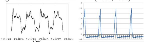
Figure 6: Bunching effect before(left) and after(right) RF optimization.
