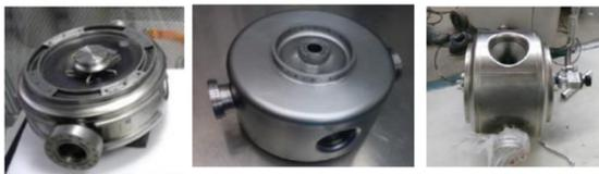
Figure 15 : S.C. Spoke cavities developed at IHEP.
