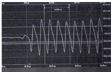
Figure 3: Measured beam rise time about 10ns after LEBT chopper.
