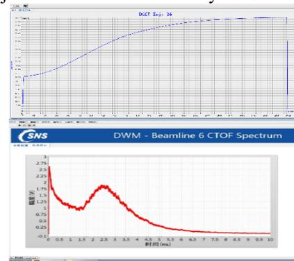
Figure 8: RCS beam transmission reached 100% (upper) and the first neutrons were generated on the target of CSNS(lower).
