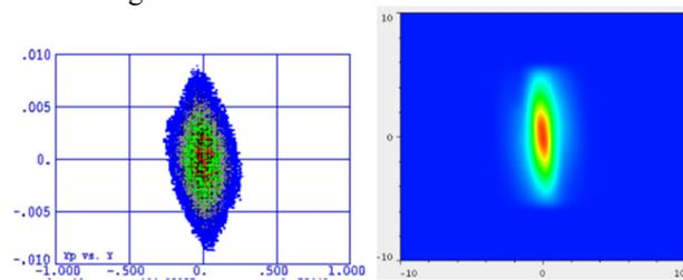
Figure 5: Simulated and measured emittance in y-direction in MEBT.
