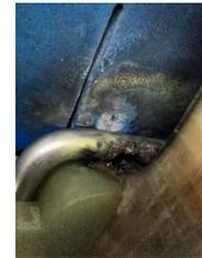
Figure 12: Discharge happened in a RCS quadrupole magnet.
