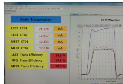
Figure 4: The best beam transmission rate of the RFQ.
