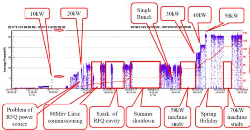
Figure 9: Overview of the beam power increase.
