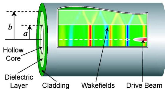
Figure 3: Conceptual drawing of the dielectric wakefield accelerator (DWA) [12],  $a = 50 \mu\text{m}$ ,  $b = 162 \mu\text{m}$ .
