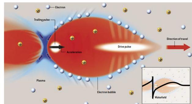
Figure 5: Conceptual drawing of the plasma wakefield accelerator [16].
