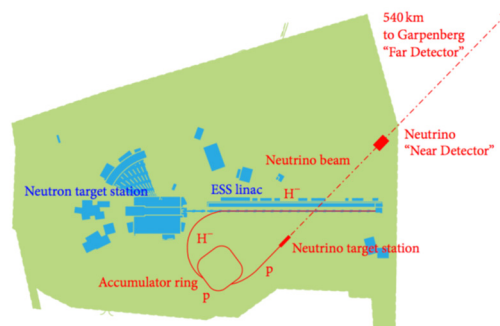
Figure 1: Layout of the ESS neutrino Super Beam facility added to the ESS neutron spallation facility.
