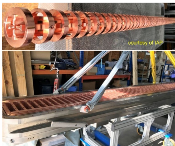
Figure 3: View on the full length ring-electrode structure (top) and the assembly of the ladder structure inside the RFQ vacuum chamber (bottom).
