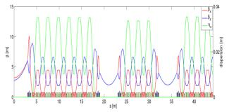
Figure 8: Symmetry 4 7BA-4BA HOA lattice (representing 1/8 of the ring).
