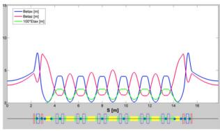
Figure 2:  $20 \times (7BA \text{ HOA lattice})$  studied in this contribution. Yellow - bends; Vertical rectangles - quads (red QD, blue QF); green - sextupoles; blue circles - octupoles.
