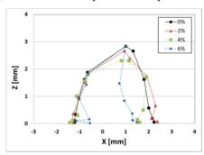
Figure 5: Dynamic aperture with 6D tracking with only single pair of chromatic sextupoles.
