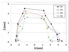
Figure 6: Dynamic aperture with 6D tracking with respectively 6 families of sextupoles and octupoles.
