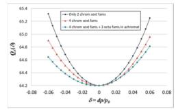
Figure 3: Horizontal momentum-dependent tune shifts for different sextupole and octupole settings.
