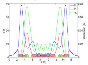
Figure 1: Baseline lattice:  $20 \times (ESRF \text{ hybrid type 7BA})$  presented in Ref. 1.
