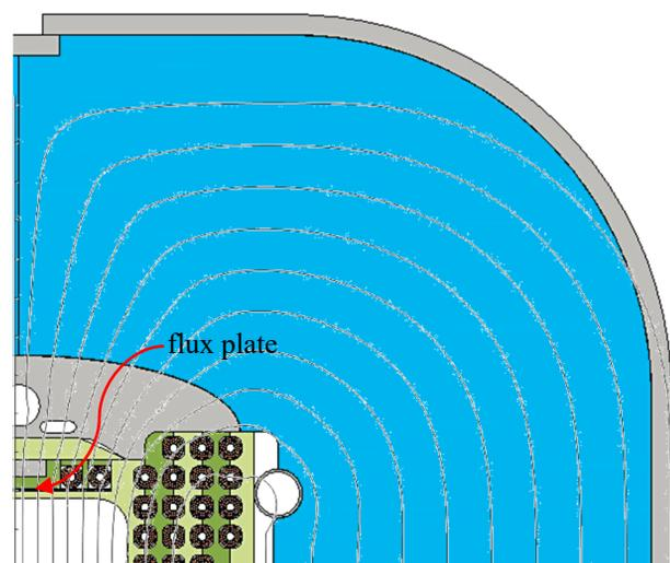
Figure 5: Quadrant cross-section of the 6 T CIC dipole: green – G-11 structure elements, blue and gray – steel flux return. Note the steel flux plate.
