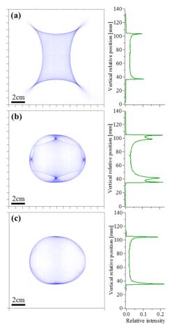
Figure 2: Spatial intensity distributions of the 10-MeV proton beam focused with one or two octupole magnets. The strengths ( $K_{OCT1}$ ,  $K_{OCT2}$ ) of the two octupole magnets are (a) (0 m<sup>-4</sup>, 3100 m<sup>-4</sup>), (b) and (c) (-10500 m<sup>-4</sup>,  $3100 \text{ m}^{-4}$ ). In (c), the beam tail has been collimated. The left and right panels are the cross-sectional and vertical axial distributions of the beams, respectively.
