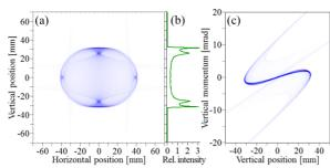
Figure 3: Tracking simulation result of the 10-MeV proton beam focused using two octupole magnets. The beam-line parameters are the same as those in Fig. 2(b). (a) Relative intensity distribution of the beam cross-section. (b) One-dimensional relative intensity distribution along the vertical axis in (a). (c) Phase-space distribution in the vertical direction.
