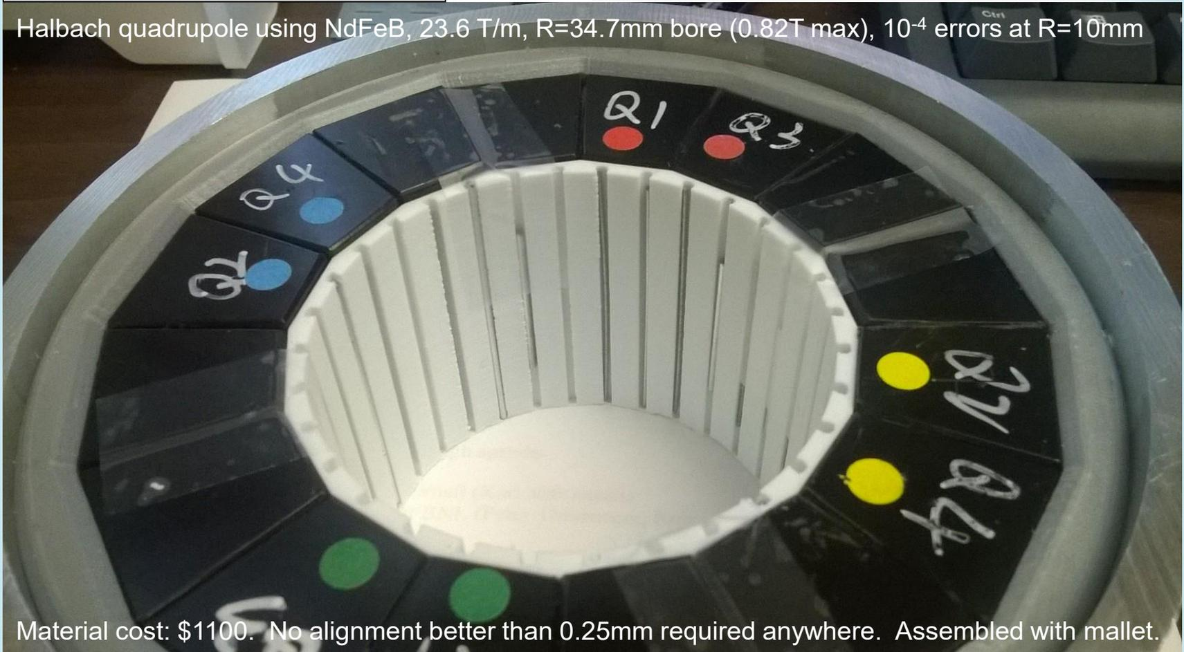
Material cost: \$1100. No alignment better than 0.25mm required anywhere. Assembled with mallet.
