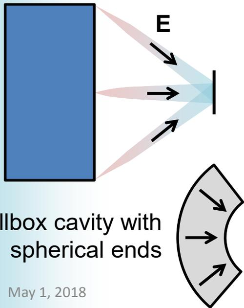
Pillbox cavity with spherical ends
