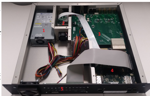
Figure 3: FRIB LLRF controller. 1. Power supply; 2. Tuner board; 3. RF board; 4. FRIB general purpose digital board (FGPDB); 5. Front panel and board.
