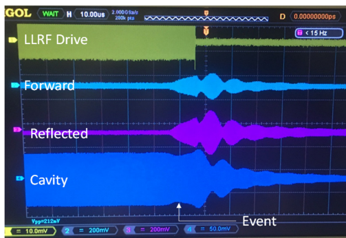
Figure 13: Before line extension. Forward power increases during spark event.
