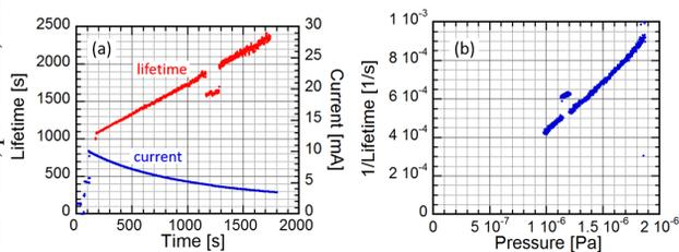
Figure 5: (a) The beam lifetime ( $\tau$  [s]) and stored current when the beam dose was 0.7 Ah. (b)  $1/\tau$  as a function of the average pressure of the arc sections.
