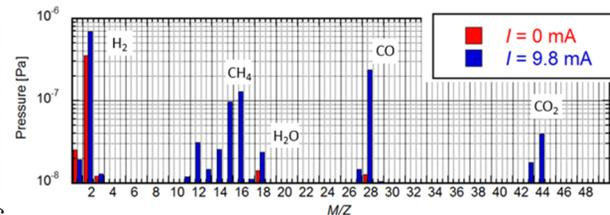
Figure 6: The mass spectrum of pressure with a beam current of 9.8 mA (average pressure:  $1.4 \times 10^{-6}$  Pa) and pressure without a beam current (average pressure:  $4.3 \times 10^{-7}$  Pa) when the beam dose was about 0.7 Ah.
