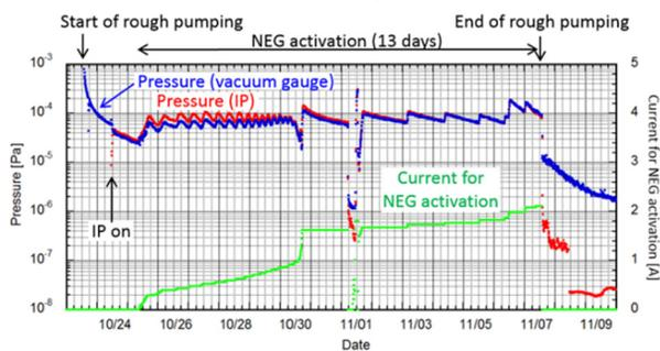
Figure 2: Pressure reading from the start of the evacuation process until the end of NEG activation in the east arc section.
