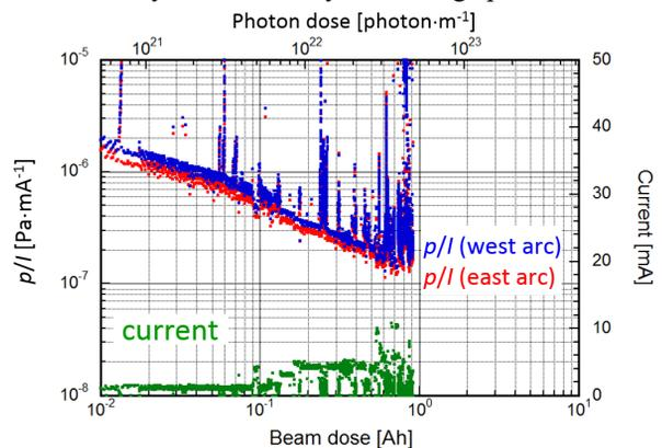
Figure 4: Average pressure normalized by a unit beam current ( $p/I$  [ $\text{Pa} \cdot \text{mA}^{-1}$ ]) for the arc sections as a function of the beam dose.
