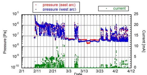
Figure 3: History of the stored beam current and the average pressure measured by the IPs of the arc sections.
