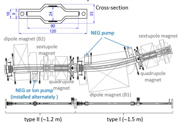
Figure 1: Two types of beam pipes for one cell of the arc sections and their cross-section.
