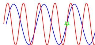
Figure 2: In heterodyne mixing a beating is looked for between two unrelated frequencies so that a common zero crossing can be found.
