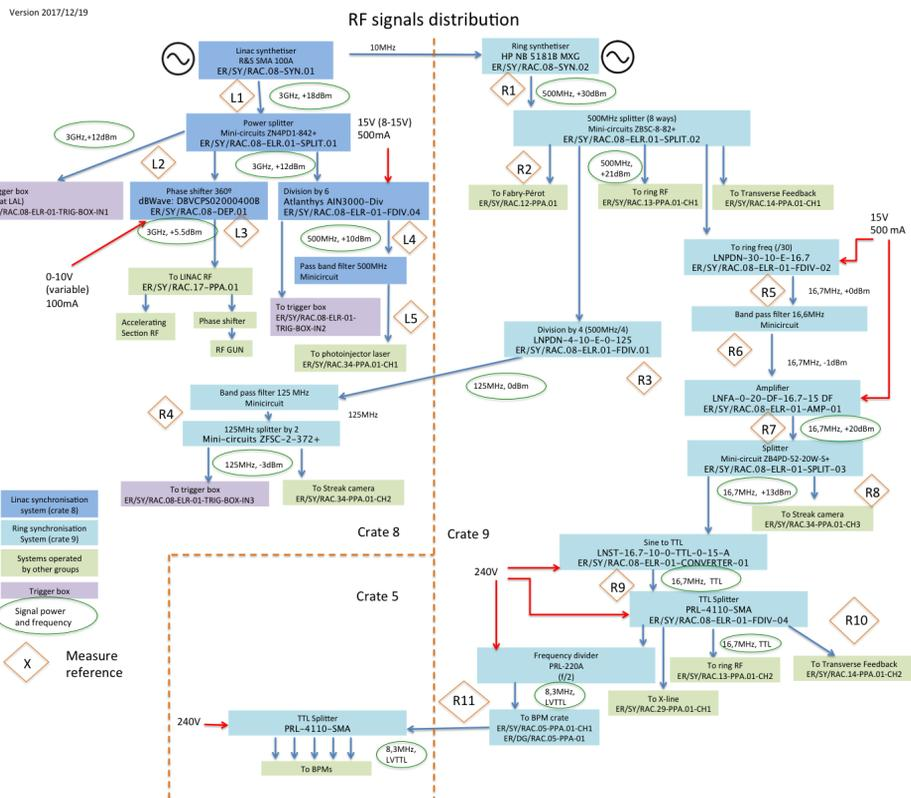
Figure 5: The RF distribution scheme.
