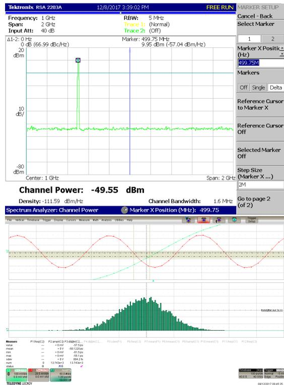
Figure 7: Measurements of the spectral purity (top) and the jitter (bottom) at point R5 of Fig. 5.
