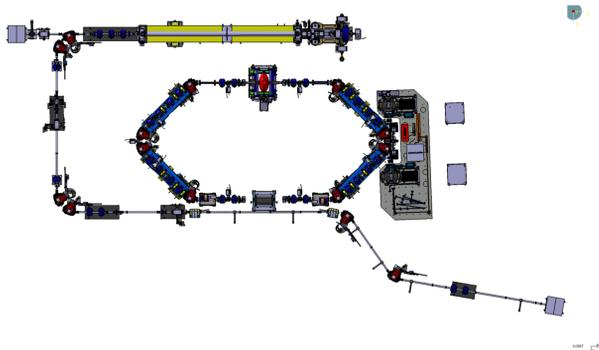
Figure 1: The ThomX compact Compton source. The linac can be seen at the top of the image, the ring in the middle and the Fabry-Perot cavity is on the right.
