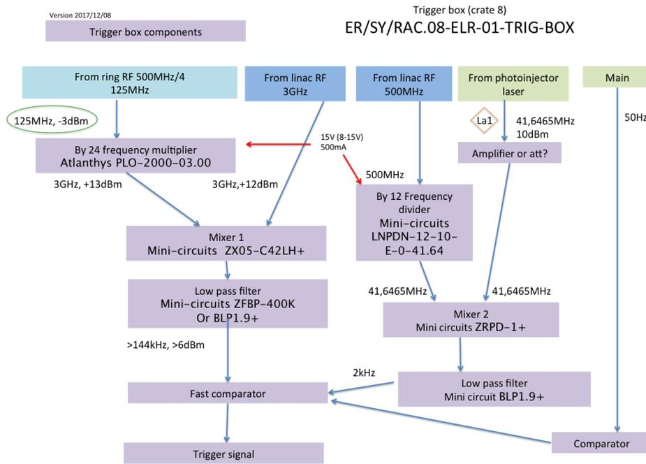
Figure 4: The frequency manipulation to find the heterodyne trigger signal.
