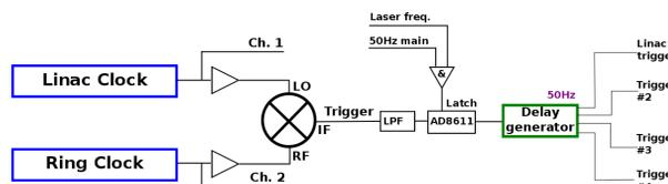
Figure 3: A simple schematic of the circuit used for zero crossing detection.
