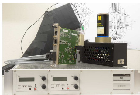
Figure 4: Wire scanner detector RTM (left) and PMT tube with base (right) standing on HV power supply. The PMT signals are connected to the RTM using differential cables with standard RJ45 connectors. In the background a black wrapped up paddle is visible partially.
