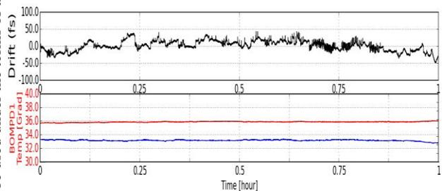
Figure 3: Out-of-loop measurement on the timing drift of the remotely generated microwave signal using the BOMPDs installed at Dalian Coherent Light Source (top). Temperature inside the BOMPD enclosure during the measurement time (bottom).
