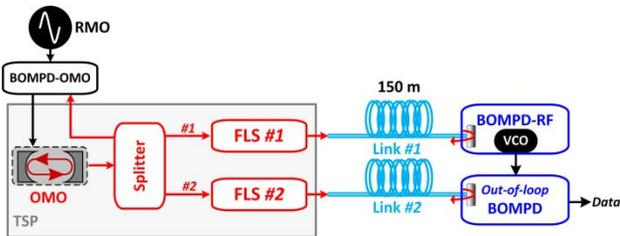
Figure 2: Measurement setup of the remote microwave generation using the BOMPDs. VCO: voltage-controlled oscillator.
