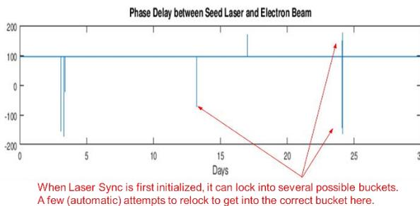
Figure 6: Coarse phase monitor of the remote seed laser compared to the electron bunch.
