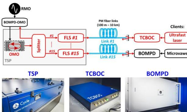
Figure 1: Layout of the timing distribution system (top sketch) and its individual modules (bottom pictures). RMO: RF master oscillator; OMO: optical master oscillator; TSP: temperature stabilized platform; FLS: fiber link stabilizer; TCBOC: two-color balanced optical cross-correlator; BOMPD: balanced optical-microwave phase detector.
