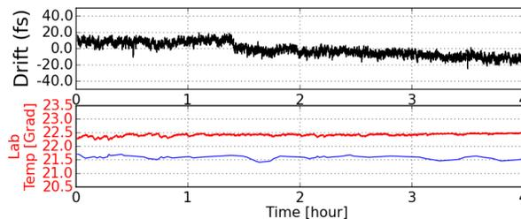
Figure 5: Out-of-loop measurement on the timing drift of the synchronized seed laser using the TCBOCs installed at Dalian Coherent Light Source (top). Temperature in the seed laser room during the measurement time. (bottom)
