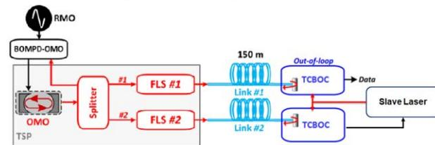
Figure 4: Performance characterization setup of the remote-station ultrafast laser synchronization using the TCBOC.
