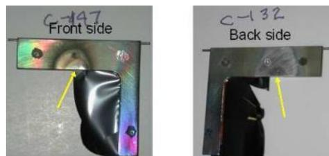
Figure 2: Used foils showing the signs of overheated frame and cracked and warped foil.
