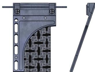
Figure 7: BL2A foil tilted at 20 deg. from vertical orientation by offsetting the frame's centre of gravity.
