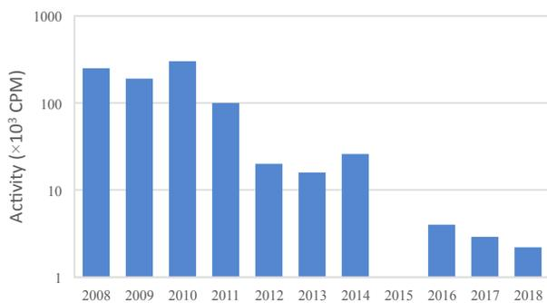
Figure 6: Cyclotron tank contamination level (7Be) under 1A foil (year 2015 data missing).
