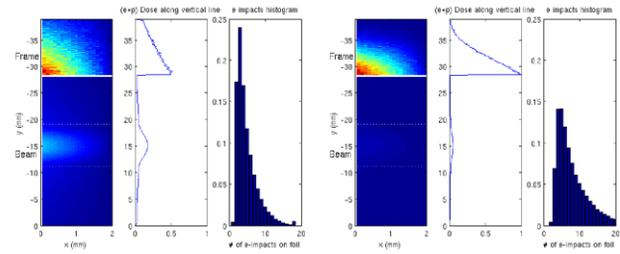
Figure 4: Results of simulation made with 5 (Left) and 1 mg/cm<sup>2</sup> (Right) foils, showing contours of energy deposit, distribution of energy deposit along y, and a histogram of number of electron impacts.
