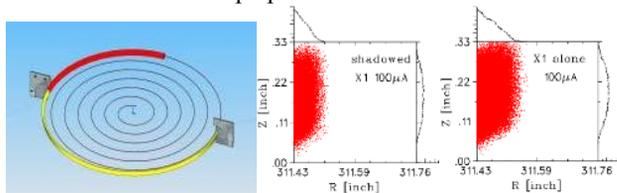
Figure 1:  $H^-$  radial shadow extraction scheme (left); simulated beam spots in the shadowed case (middle) and in single foil case (right). The spot size is  $\sim 2 \times 8$  mm.
