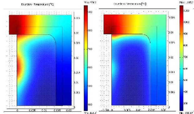
Figure 5: The foil (PG) and frame (SS) temperature distribution, calculated with 5 (Left) and 1 mg/cm<sup>2</sup> (Right) thicknesses. The darkest red is 1100C.
