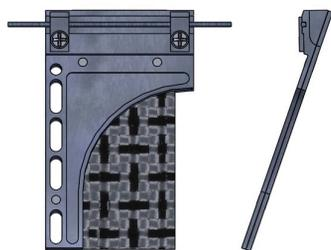
Figure 7: BL2A foil tilted at 20 deg. from vertical orientation by offsetting the frame's centre of gravity.
