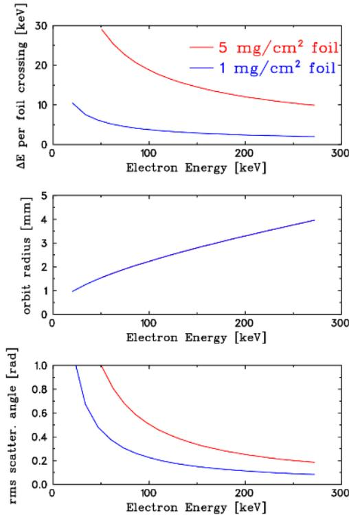
Figure 3: Top-to-bottom: Stripped electron energy drop per foil crossing, electron precession orbit radius in Bz, electron rms scatter angle vs electron energy for two typical foil densities: 1 & 5 mg/cm<sup>2</sup>.
