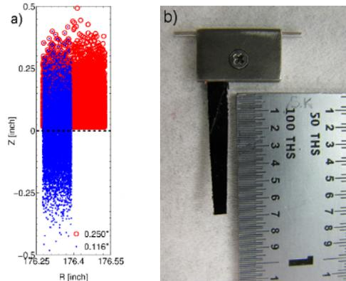
Figure 8: a) Particle distribution on fully (blue) and partially (red) dipped foils with the same split ratio 0.4; foils widths are 0.116" and 0.250" respectively. b) BL2C4 extraction "wedged" foil.
