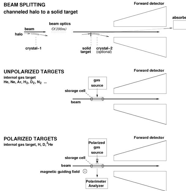
Figure 1: Sketches of three fixed target setups: crystal beam splitting for a double-crystal setup (top) and unpolarized (middle) and polarized (bottom) gaseous targets.
