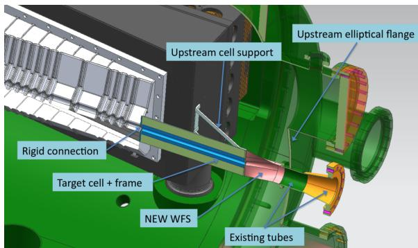
Figure 4: A proposed implementation of an openable storage cell in LHCb to increase the unpolarized gas target thickness. Only one half is shown, for clarity. Courtesy of V. Carassiti (INFN Ferrara).
