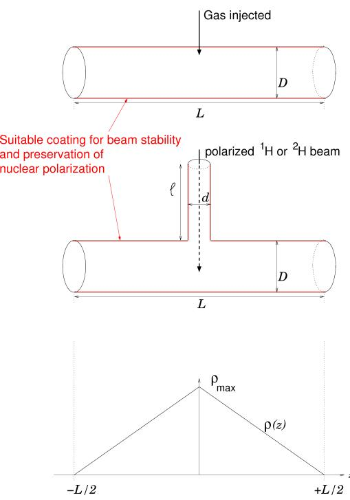
Figure 3: Principle of storage cell with triangular gas distribution (see e.g. [31]). Top: typical situation for unpolarized gas (or polarized  $^3\text{He}$ ). Middle: the case with a feed tube for an atomic beam ( $^1\text{H}$ , D). Bottom: resulting density profile along the beam axis.
