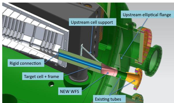
Figure 4: A proposed implementation of an openable storage cell in LHCb to increase the unpolarized gas target thickness. Only one half is shown, for clarity. *Courtesy of V. Carassiti (INFN Ferrara).*
