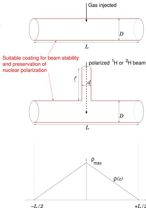
Figure 3: Principle of storage cell with triangular gas distribution (see e.g. [31]). Top: typical situation for unpolarized gas (or polarized  $^3\text{He}$ ). Middle: the case with a feed tube for an atomic beam ( $^1\text{H}$ ,  $\text{D}$ ). Bottom: resulting density profile along the beam axis.
