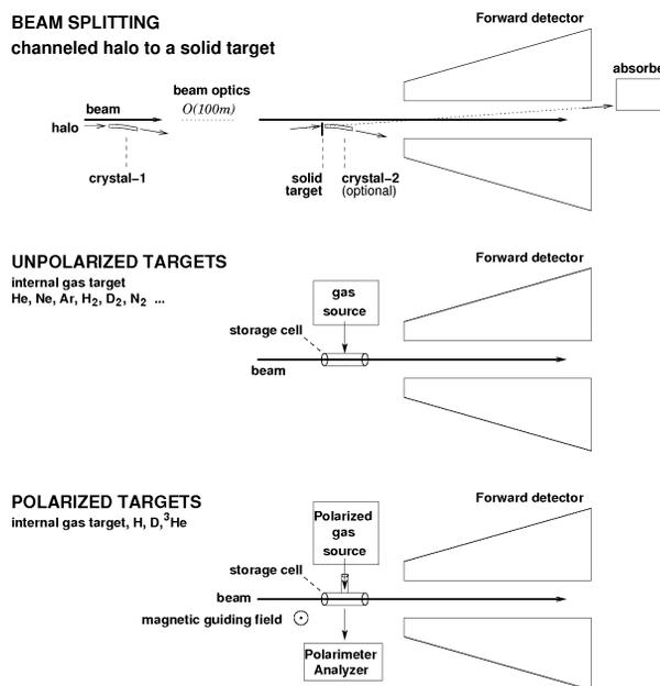
Figure 1: Sketches of three fixed target setups: crystal beam splitting for a double-crystal setup (top) and unpolarized (middle) and polarized (bottom) gaseous targets.
