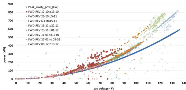
Figure 7: Plot of the forward power vs cavity voltage during RFQ conditioning. The blue curve represents nominal relation in case of RFQ quality factor. At high voltage, more power than nominal one is required to reach the nominal field because the pulse duration was lower than the one needed to establish flat-top cavity field.
