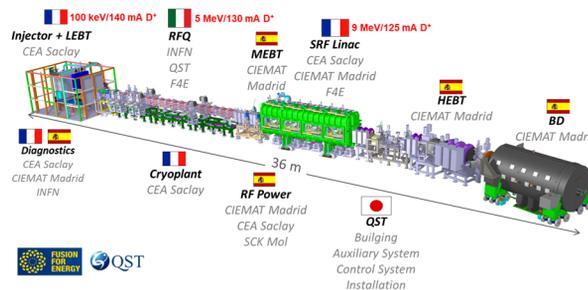
Figure 1: Linear IFMIF Prototype Accelerator.
