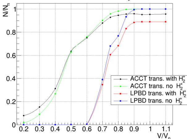
Figure 3: Simulated proton transmission from the RFQ with respect to different voltage ratios at the MEBT ACCT and the LPBD. The two curve ensembles are related to the calculations with and without contaminants.
