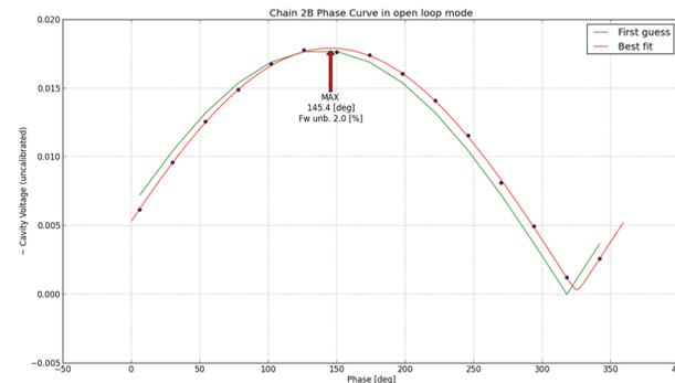
Figure 6: Chains phasing in general case of power unbalance. The curve minimum is obtained with couplers powered at  $180^\circ$  reciprocal phases. When power levels are perfectly balanced this will result in zero power into RFQ.
