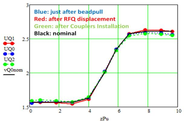
Figure 5: Evolution of the RFQ voltage along installation phases.
