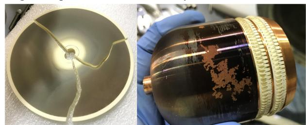
Figure 9: Damaged RF window (on the left) showing a strong deposition that subsequent analyses revealed to be copper deposition. Anchor connector (on the right) bolted on the alumina window experienced a lot of uncontrolled arcs that removed copper from surface and sputtered alumina surface itself.
