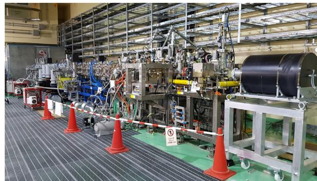
Figure 2: LIPAc phase B configuration (2.5 MeV/u pulsed). Low power beam dump, diagnostic plate, MEBT, RFQ, LEBT and source can be seen.
