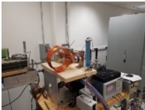
Figure 3: Pi-Circuit extraction resonator and the low power IOT electron gun at NRL. The inductor is made of copper tubing and the capacitors of the pi-circuit sits on top of the IOT gun.
