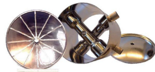
855 MHz, \beta_0=0.30 , 2-gap spoke resonator
