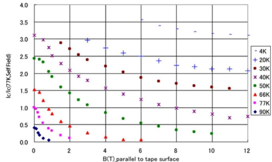
Critical current depends on the operating temperature and the strength and direction of magnetic field on the tape surface. They are scaled by  $I_c$  at 77K and with self field.
