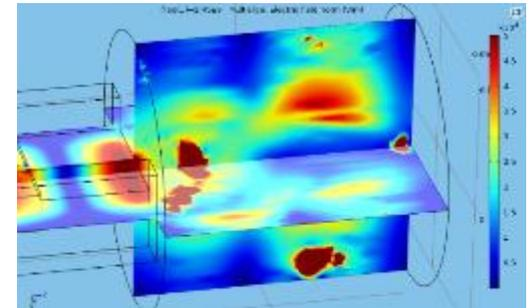
*G. Torrasi et al. "Full-wave FEM simulations of electromagnetic waves in strongly magnetized non-homogeneous plasma", JEWA 2014 vol. 20, no. 9, 1085-1099*
