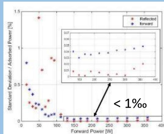
Measured forward and reflected pulsed power
