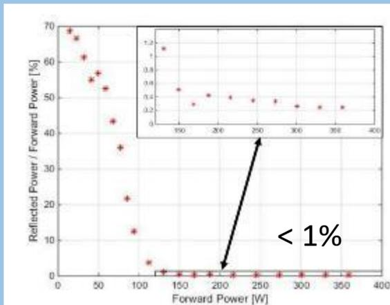
High measured stability of forward and reflected power
