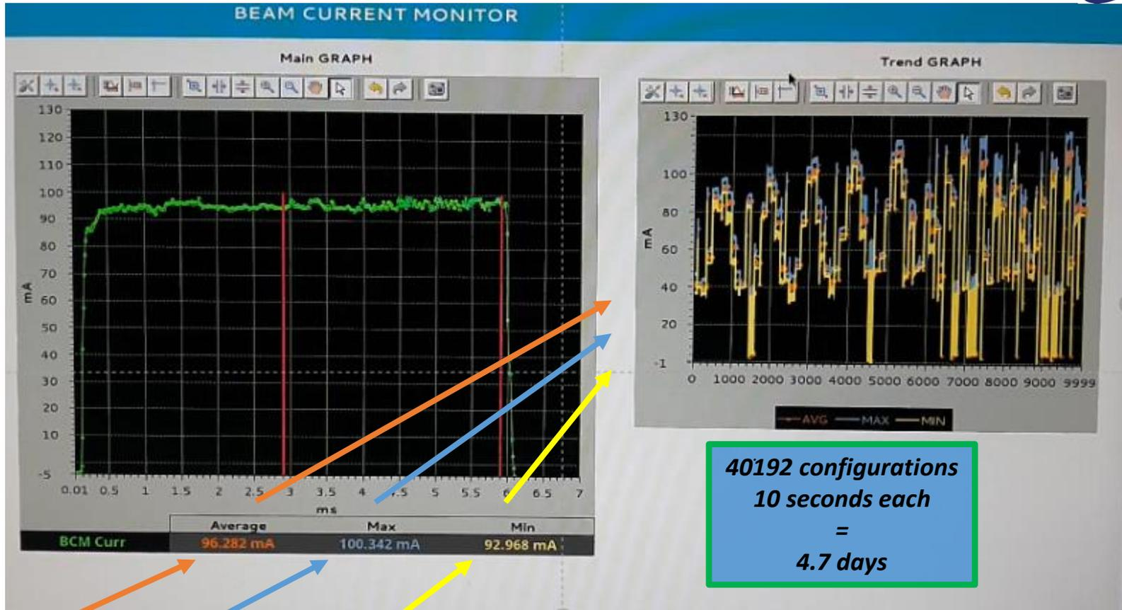
In the graphical interface: **average**, **maximum** and **minimum** are evaluated and the trend showed for the beam pulse between 2.9 ms and 5.9 ms .
