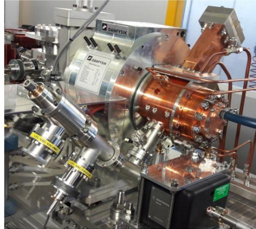
This required the development of an high gradient/high rep. rate photo-gun operating at 120 MV/m cathode peak field
