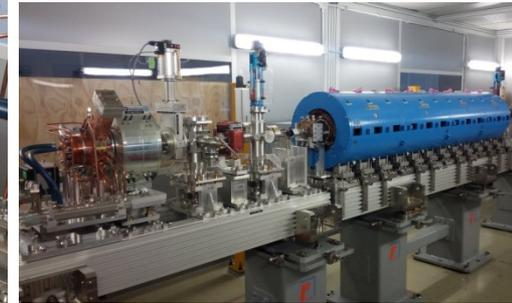
This required the development of **special damped C band cavities** operating at 33 MV/m
