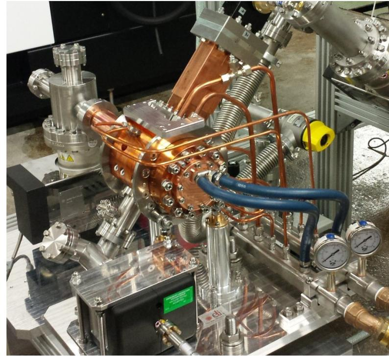
Final assembly in **clean room**. The gun has been **vacuum leak tested**, then **measured at RF and tuned** (acting on deformation tuners) at low power. Finally, assembled with **cooling system and support**.
