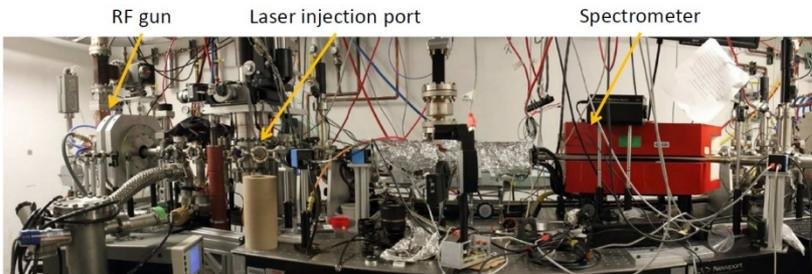
*UCLA Pegasus lab with clamped RF gun in operation (90 M/m 5 Hz)*
