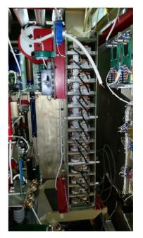
Figure 1: Final Power Amplifier High Voltage Switch Assembly. Switch consists of 14 IGBT switch plates and incorporates thick copper baseplates for inertial.
