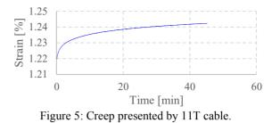
Test Protocol 3 confirmed the viscoelastic nature of Nb3Sn superconducting cables.
