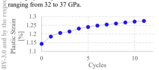
Figure 4: Plastic deformation after load-unload cycles in 11T azimuthal cables.
