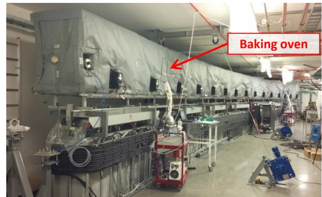
Figure 2: 3 GeV storage ring vacuum system baking oven.
