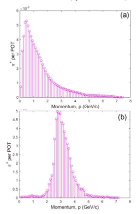
Figure 4: Momentum distribution (a) before PMAG and, (b) after the PMAG. PMAG selects particles near 3.1 GV/c.
