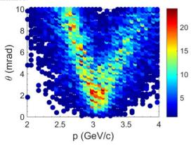
Figure 5: Pion momentum as function of the transverse angle after the beam passes the pulsed magnet. Particles near 3.1 GeV/c have the lowest possible transverse angle.
