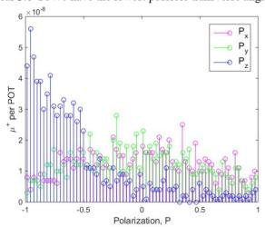
6: Vertical, horizontal and longitudinal components of polarization just upstream of PMAG. The average polarization in the longitudinal direction is 0.55. The average polarization in the horizontal and vertical planes is near zero.
