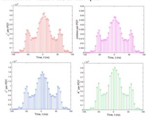
Figure 3: Longitudinal profiles of the secondary beam after it exits the Lithium lens (upstream of PMAG).
