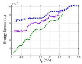
Figure 3: Energy spread vs single bunch current calculated from SLM camera bunch size measurements for the three different lattices BL, 1DW and 3DW at  $V_{RF}$  = 2.6MV.
