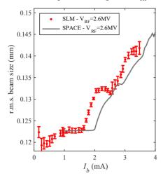
Figure 6: Horizontal beam size change as a function of single-bunch current for the 3DW lattice at RF voltage  $V_{RF} = 2.6MV$ .
