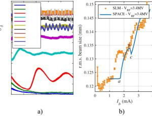
Figure 4: SPACE simulations for 3DW lattice and comparison with SLM measured data at  $V_{RF} = 3.4 MV$ . a) Turn-by-turn energy spread for different values of singlebunch current. b) Horizontal beam size change as a function of single-bunch current. Orange dots with error bars are SLM data and the blue trace is the maximum amplitude (over the last 5000 turns) of the energy oscillations from Fig. 4a.
