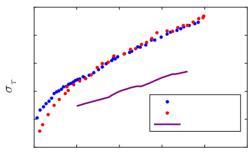
Figure 7: Bunch lengthening dependence on single-bunch current  $I_b$ . Comparison of numerical simulations vs measured results made by the streak camera at  $V_{RF} = 3.4MV$  for bare lattice and for regular operational lattice with 3DWs magnet gap closed.
