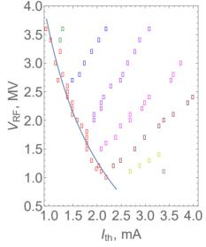
Figure 8: Summary of the measured single-bunch instability thresholds at different RF voltages. Red dots represent the first microwave instability threshold behavior. Blue curve is a fit to  $1/\sqrt{V_{RF}}$ .
