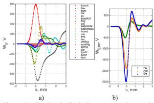
Figure 2: The longitudinal short-range wakepotential calculated for a  $\overline{\sigma}_s = 0.3mm$  bunch length. a)  $W_{||}(s)$  calculated for each individual vacuum component and multiplied by a total number. b) The total longitudinal wakepotential  $W_{||,tot}(s)$  of the NSLS-II storage ring as a sum of geometric and resistive wall wakepotentials.
