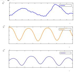
Figure 5: Zoomed part of the energy oscillations from Fig. 4a for three highlighted regimes shown on Fig. 4b: a)  $I_b = 1.65mA$  blue trace, b)  $I_b = 2.35mA$  orange trace and c)  $I_b = 2.5mA$  dark blue trace.
