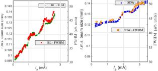
Figure 1: Horizontal beam size change measurements from SLM camera and FWHM measured form the IVU spectrum of  $7^{th}$  harmonic at  $V_{RF} = 2.6MV$  for the two different lattices BL and 3DW.
