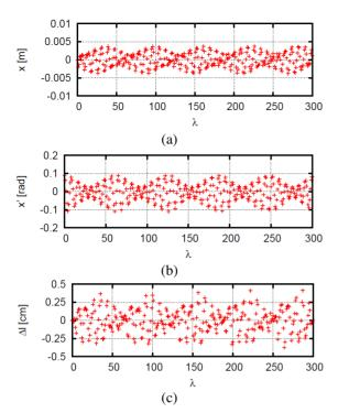
Figure 3: (a) Transverse position x in the absorber plane over 300 periods in the Skew PIC channel with no damping effects included. (b) Transverse angle x'. (c) Path length difference  $\Delta l$ .
