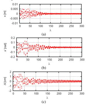
Figure 4: (a) Transverse position x in the absorber plane over 300 periods in the Skew PIC channel with damping effects included. (b) Transverse angle x'. (c) Path length difference  $\Delta l$ .
