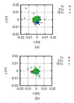
Figure 1: (a) x-y phase space in the absorber plane after 1, 51, and 101 periods of the single sextupole-decapole channel. (b) x-y phase space in the independently-varying sextupole and octupole channel.
