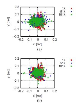
Figure 2: (a) x'-y' phase space in the absorber plane after 1, 51, and 101 periods of the single sextupole-decapole channel. (b) x'-y' phase space in the independently-varying sextupole and octupole channel.
