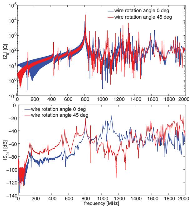
Figure 6: Wakefield simulation (top) and probe-to-feed-through transmission measurement results (bottom) for the wire rotation angles of 0 and 45 degrees respectively.
