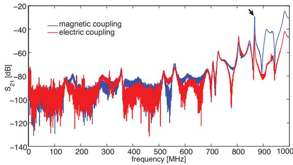
Figure 5: Probe-to-wire measurement results to quantify the relative electric and magnetic coupling of the EM-modes.
