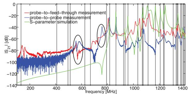
Figure 4: Comparison between simulated measurement and probe-to-probe as well as probe-to-feed-through measurement for a 0 degrees rotation angle of the wire. The vertical black lines indicate the frequencies found by the CST [9] eigenmode solver and the oval frames enclose probe modes which occur as an artifact of the measurement.
