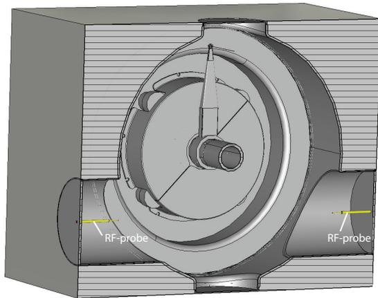
Figure 2: CST EM simulation model for S-parameter calculation of the probe-to-probe measurement. Note the axial position of the RF-probes and that the tip of the probe couples only to electric fields with non-zero field component at the axis.
