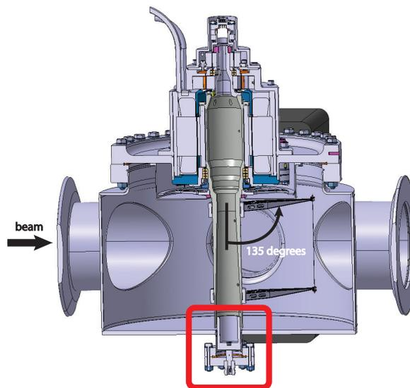
Figure 1: 3D CAD model of the PSB wire scanner in cross-sectional view. The fork is positioned in a 135 degrees rotation angle with respect to the so-called parking position (0 degrees) and the capacitive rod coupler and air-side N-connector are highlighted with a red frame.
